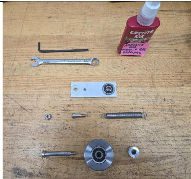
1. Install the Bearing, 42001245 use Loctite#638 around the bearing
