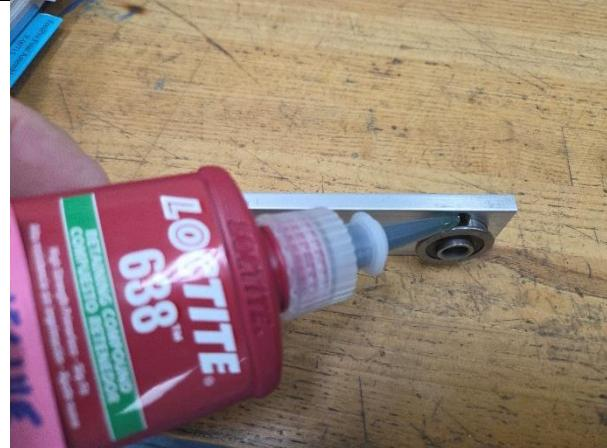
2. Install the Wheel to the Bar (Note that it is on the SAME side as the flange of the bearing.)
